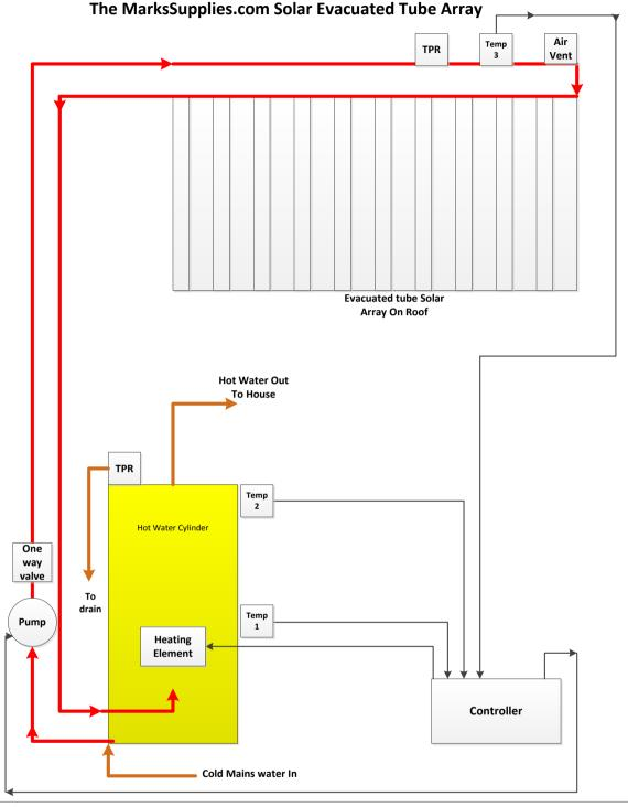
Before the solar installation the cylinder had just a cold water in and a hot water out shown in orange, above we have added 2 extra pipes to the cylinder shown in red, one to take cold water from the bottom of the cylinder to the evacuated tubes and the second to bring the hot water back down & into the cylinder.
